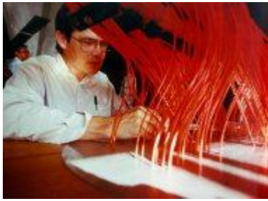
Plugging spectrograph fibers into the pre-drilled plate
