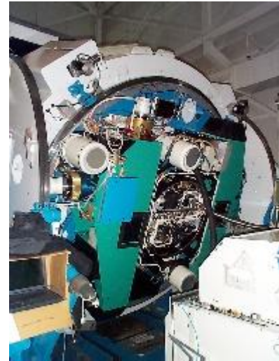
The back side of the telescope, with the main camera (center, black) and the two spectrographs (green boxes). Click for a larger image.
